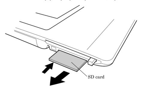
Figure 4-3 Removing the SD card
